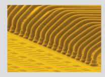
COR mils) - Wire bonder: K65 90285 - Package (O.8 mils) - Wire bonder: K65 90285 - Package (O.8 mils) - Wire spans : 3.5 - 4.5 mm Loop Height Range. 150-165 µm · Bonding
