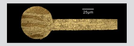
These highly doped wires of different chemical compositions are very suitable for low and long loop applications. Both wire types are comparable in their characteristics and offer outstanding material and processing properties as well as good high temperature strength.
