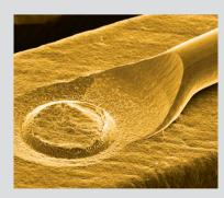
Bonding Conditions: Wire diameter: 33 µm · Wire bonder: K8S 1488 turbo Package type: PLCC 68 leads · Die metallization: AISi (1%) Ou (0.5%) Leadranne: Ag: Plated Cu. Wire span: 3.2 – 4 mm · Loop height range: 30 µm +/-Ronding remnerature: 240°C: Caullava, 41.43–401.3-37 mil R R 9°
